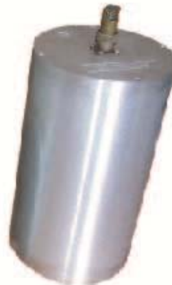
Motion reference unit mounted under the flight deck.
